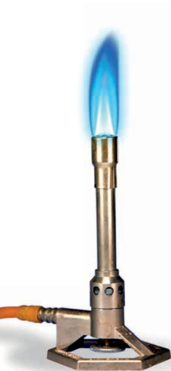
▲ The Bunsen burner controls the combustion of methane, \text{CH}_4 , and is often used as a source of heat in the laboratory.
