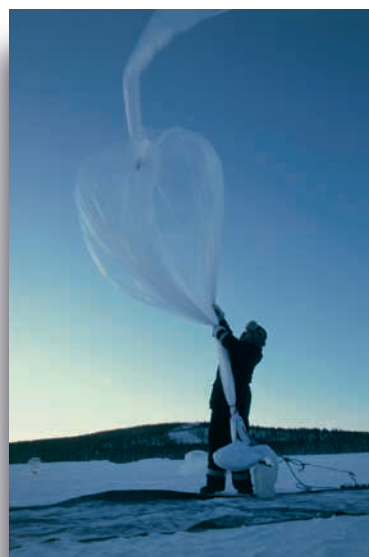
▲ Technician releasing a balloon to measure stratospheric ozone over the Arctic. This research was part of a joint project by NASA and the European Union to look at the amount and rate of stratospheric ozone depletion.
